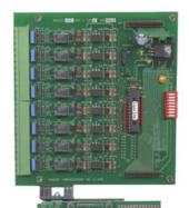
The EAC800 Elevator Access Controller incorporates application firmware and a LONWORKS® control module. As a member of The Smart Touch® Product Family, EAC800 is fully compatible with Habtech ST2000 Security Management Systems.
